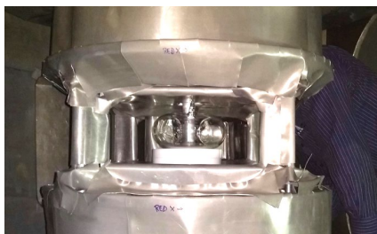
JCNS PASTIS on NEAT showing the cryostat and ^3\text{He} PASTIS cell installed providing large scattering angles.
